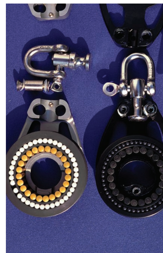
These modern blocks use a combination of ball bearings and roller bearings. Spreading the load means less friction and less wear and tear on each bearing.
