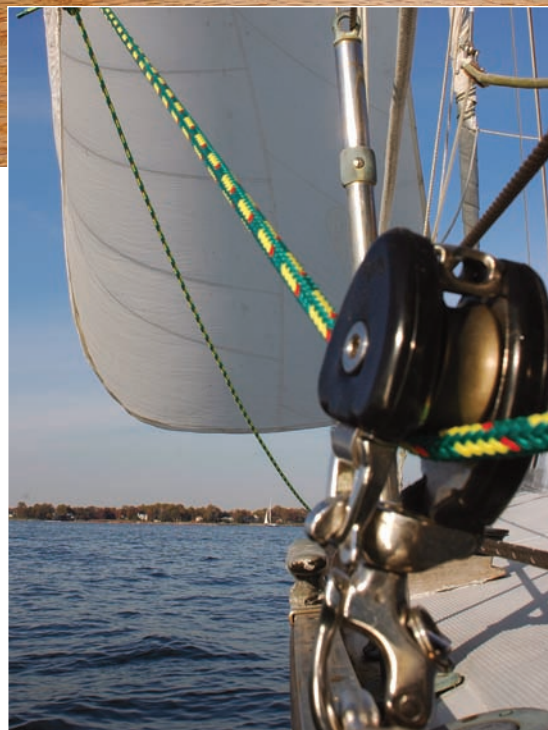
Above, snatch blocks come in a variety of sizes and styles. They come in handy for changing jib sheet angles.
