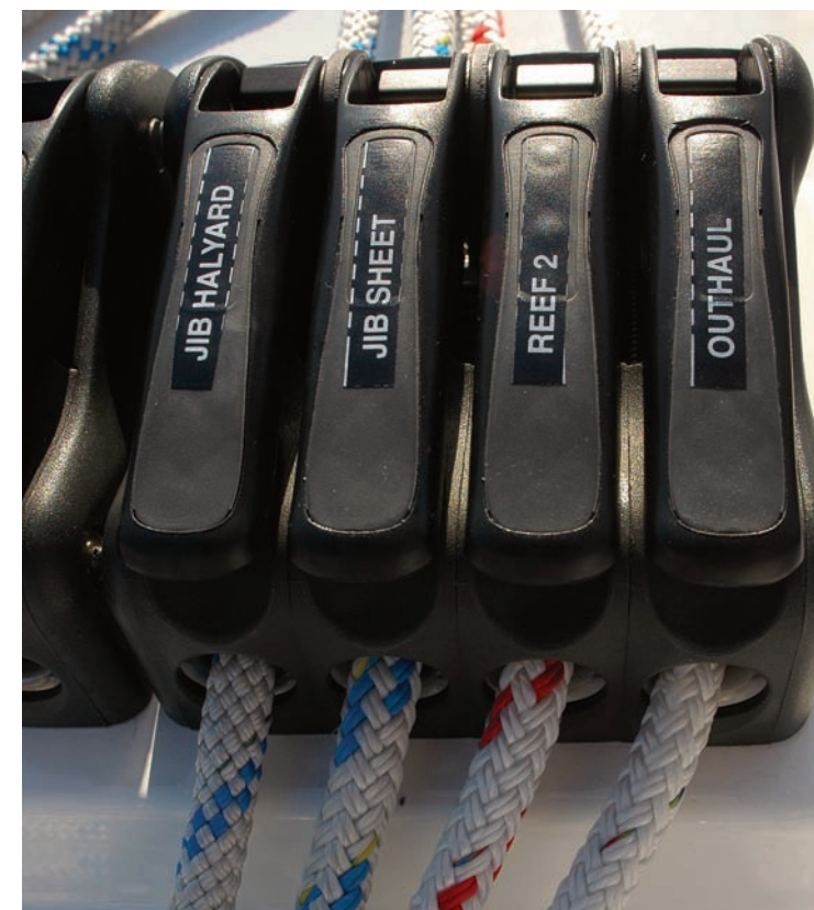
When most lines are led aft, rope clutches allow one or two winches to handle numerous jobs.
